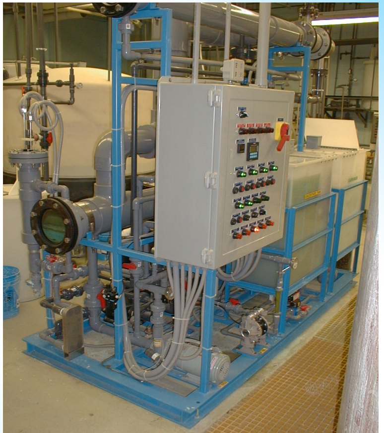
50 Gal per hour single effect vacuum evaporator used for the distillation of wastewater from aircraft component manufacturing operations
