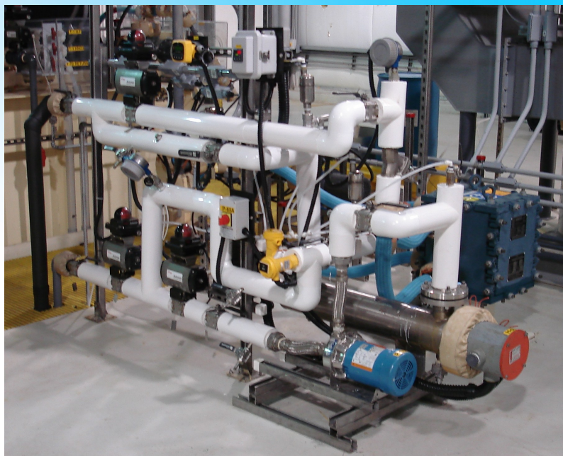
Heating/Cooling system for controlling temperature of hydrofluoric (HF) acid/nitric (HNO 3 ) acid chemical milling bath. Heat exchanger is Teflon impregnated graphite.
