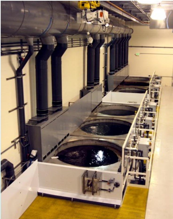
Acid etching system for aircraft parts and components
