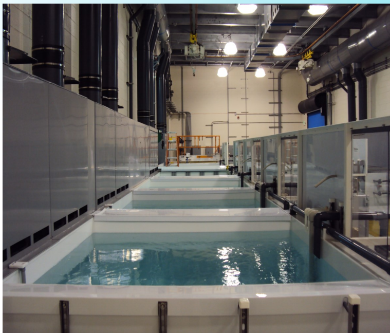
Alkaline cleaning and etching systems for aircraft and turbine parts & components
