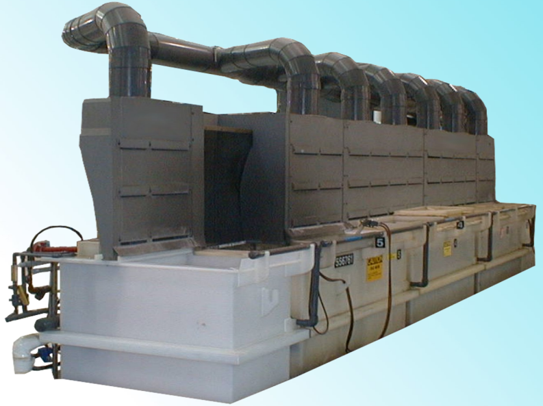
Hydrochloric acid stripping operation for blades and vanes for jet engines
